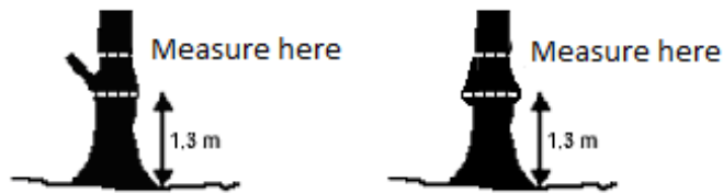
Figure 6: Dbh measurement position for a tree with branch enlargement at 1,3 m
