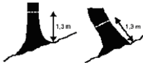
Figure 2: Dbh measurement position for a tree on steep terrain.
